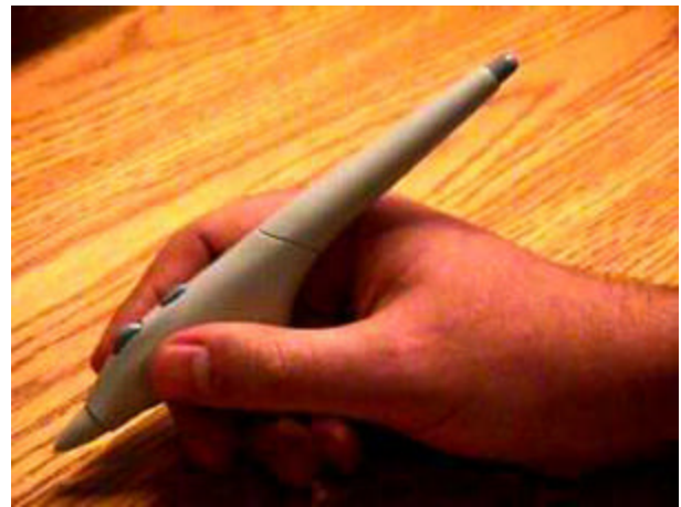
Figure 3: The Stylus Pen and its various elements: the eraser (on top), the tip, on bottom and the wheel, close to the index finger.
