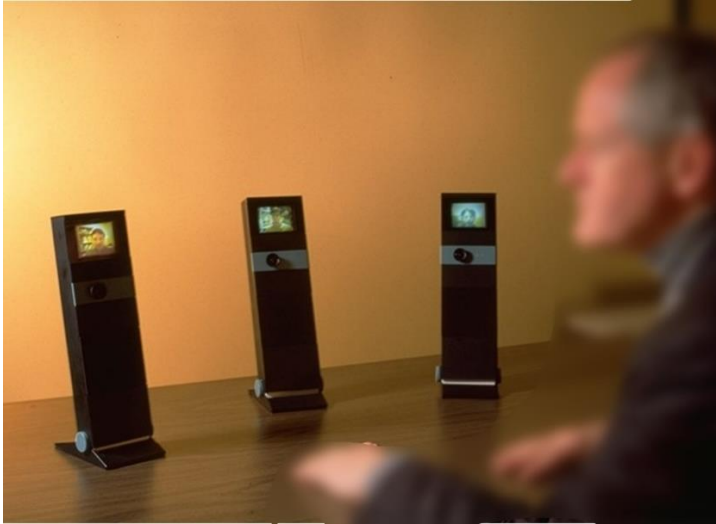
Figure 4: A 4-way round-the table conversation. By dedicating Hydra unit for each person, each occupies their own personal space at the virtual table. Their Hydra's camera constitutes their surrogate eyes, its speaker their surrogate mouth, and its microphone their surrogate ears. By preserving the "round-table" relationships illustrated schematically on the right, conversational acts found in face-to-face meetings, such as gaze awareness, head turning, etc. are preserved
