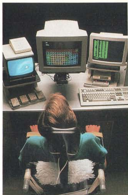
A nonintrusive eye tracker. A video camera mounted under the display tracks the position of the eye's pupil and translates the data into screen coordinates. Thus, the eyes can "point." (Photo courtesy of L.C. Technologies, Fairfax, VA)
