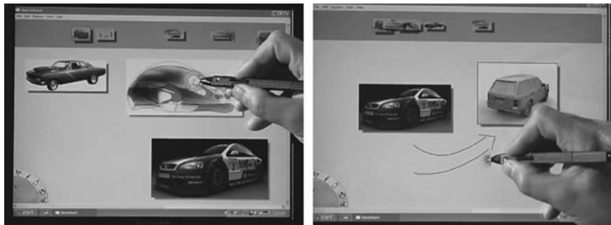
Figure 21. Working on Sketchboard from the TabletPC. (Left) using tracking menu; (right) drawing directly on the board (via the TabletPC).
