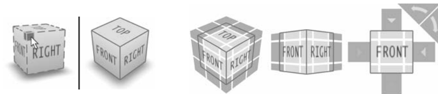
Figure 17. (Left) Before and after clicking the highlighted corner. (Right) Expanded hit areas for boundary buttons. Clicking anywhere within the green regions will select the corresponding button.
