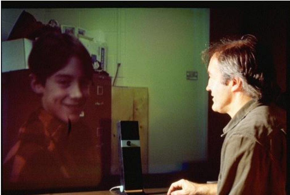
Fig. 13. 9 Face-to-Face. In this scenario, each participant has a computerized desktop on which the same information is displayed. The intention is to capture the essence of working across the desk from one-another. Each sees the remote participant life-size. The video camera (from a Hydra unit) is unobtrusive on the desk. Participants interact with the computer using a stylus. When one participant looks down to their desktop, their eyes seem to project into the space of the other, thereby strengthening the sense of telepresence. While there is a considerable amount of technology involved, it is integrated into the architectural ecology. What one gets is lots of service and lots of space, not lots of gear and appliances.
