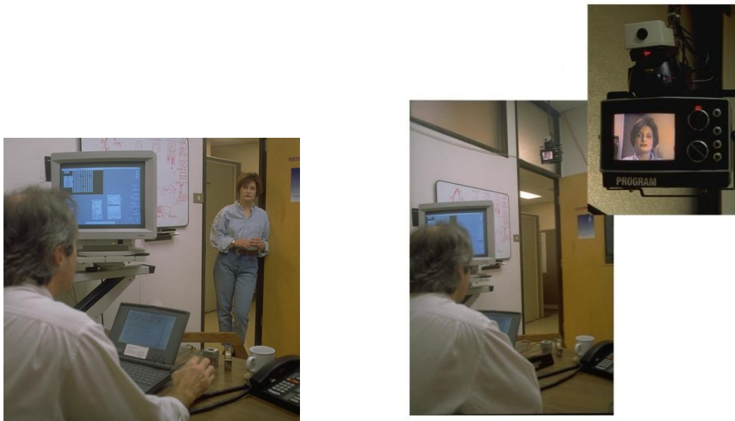
Fig. 13. 4 Maintaining Social Distance. In establishing contact, one appears by the door and has a from-the-door view via the camera, regardless of whether one approaches from the physical corridor (left image) or the electronic corridor (right image). People approaching electronically do so via a monitor and speaker mounted above the door (inset on right image). The social graces of approach are preserved, and the same social conventions are used for both physical and electronic visitors.
