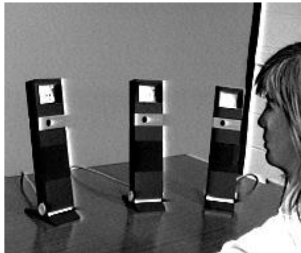
Figure 4: A user is seated in front of three Hydra units. In the photo, the Hydra units sit on the table in the positions that would otherwise be occupied by three remote participants. Each Hydra unit contains a video monitor, camera, and loudspeaker. A single microphone conveys audio to the remote participants (From Buxton & Sellen, 1991).
