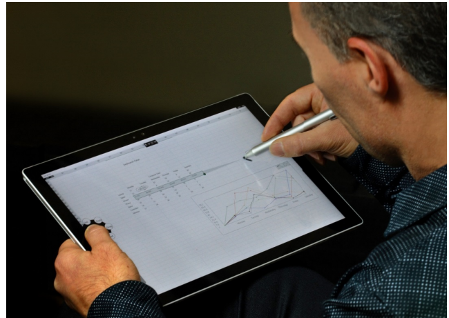
Figure 1: Thumb + Pen interaction enables simultaneous bimanual pen+touch while holding a tablet with the off-hand.
