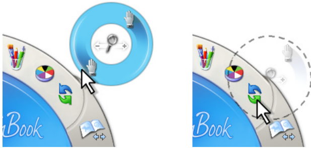
Figure 12. Pan-and-zoom tracking menu under tool palette with x-ray feedback.
