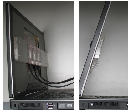
Figure 7: Side views of the prototype ThinSight laptop – note that the screen has been reversed in a ‘tablet PC style’. The only noticeable increase in display thickness is due to the acrylic plate which we plan to replace with a much thinner alternative.
