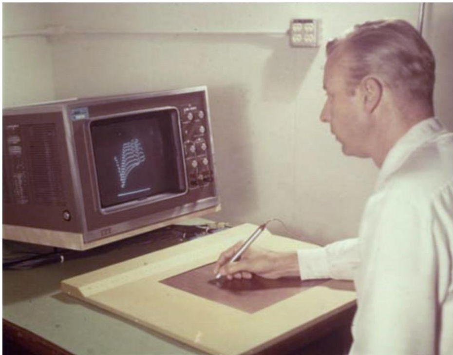
Figure 6: Tom Ellis, one of the inventors, using the RAND tablet. In his right hand is the tethered stylus, and on the screen a series of graphic lines. (Photo: Computer History Museum Collection, Catalog Number: 102710338). (Note: need to secure permission.)
