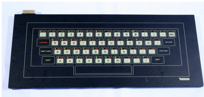
Figure 2: The Writehander (NewO Co.): a chording keyboard for one-handed text entry.
