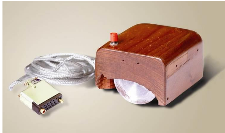
Figure 5: The Original Mouse by Engelbart and English.
