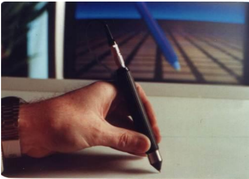
Figure 8: A Tilt-Sensing Stylus (GTCO Corp)
