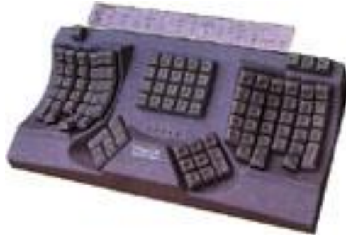
Figure 1: The Maltron keyboard: radical design sculpted to fit shape of hand and fingers.
