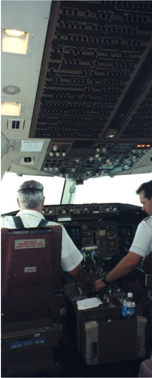
Figure 6: Space Multiplexed Controls: an Aircraft Cockpit
