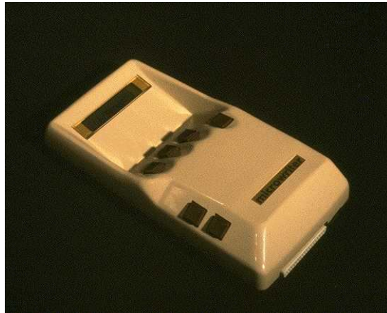
Figure 13: Key Layout Preventing Left-Handed Operation (Microwriter Ltd.)
