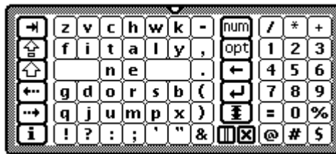
Figure 16: The Fitaly One-Finger Keyboard as it appears on the Newton MessagePad
