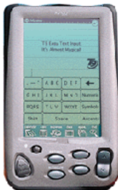
Figure 17: The T9 Graphical Keyboard on the Texas Instruments' Avigo PDA.
