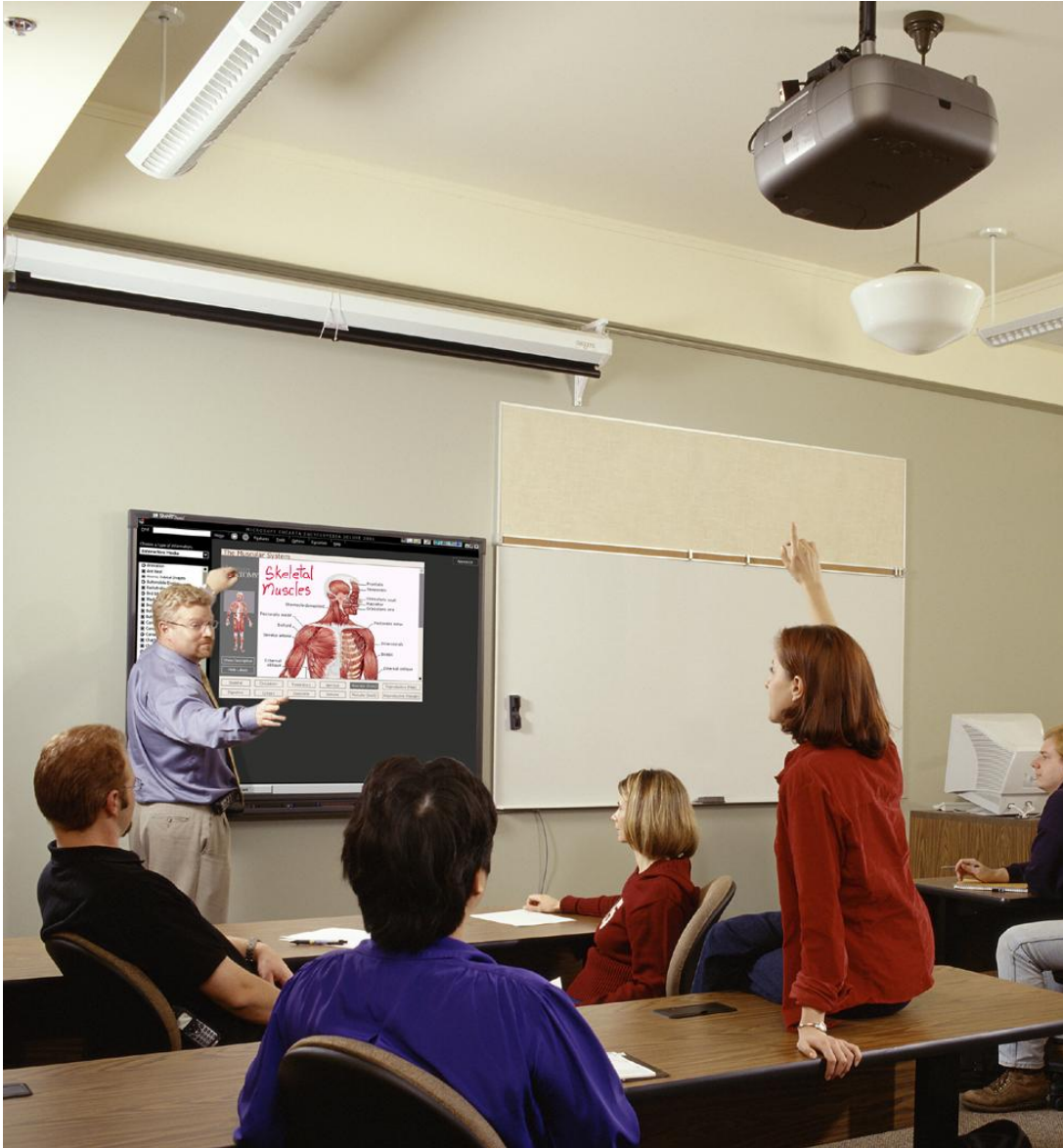
Figure 9: Electronic Whiteboard: The camera system shown on the right is used to capture information on and interactions with the whiteboard. The projection system can be used to project data onto whiteboard. (Image: SMART Technologies, Inc.).
