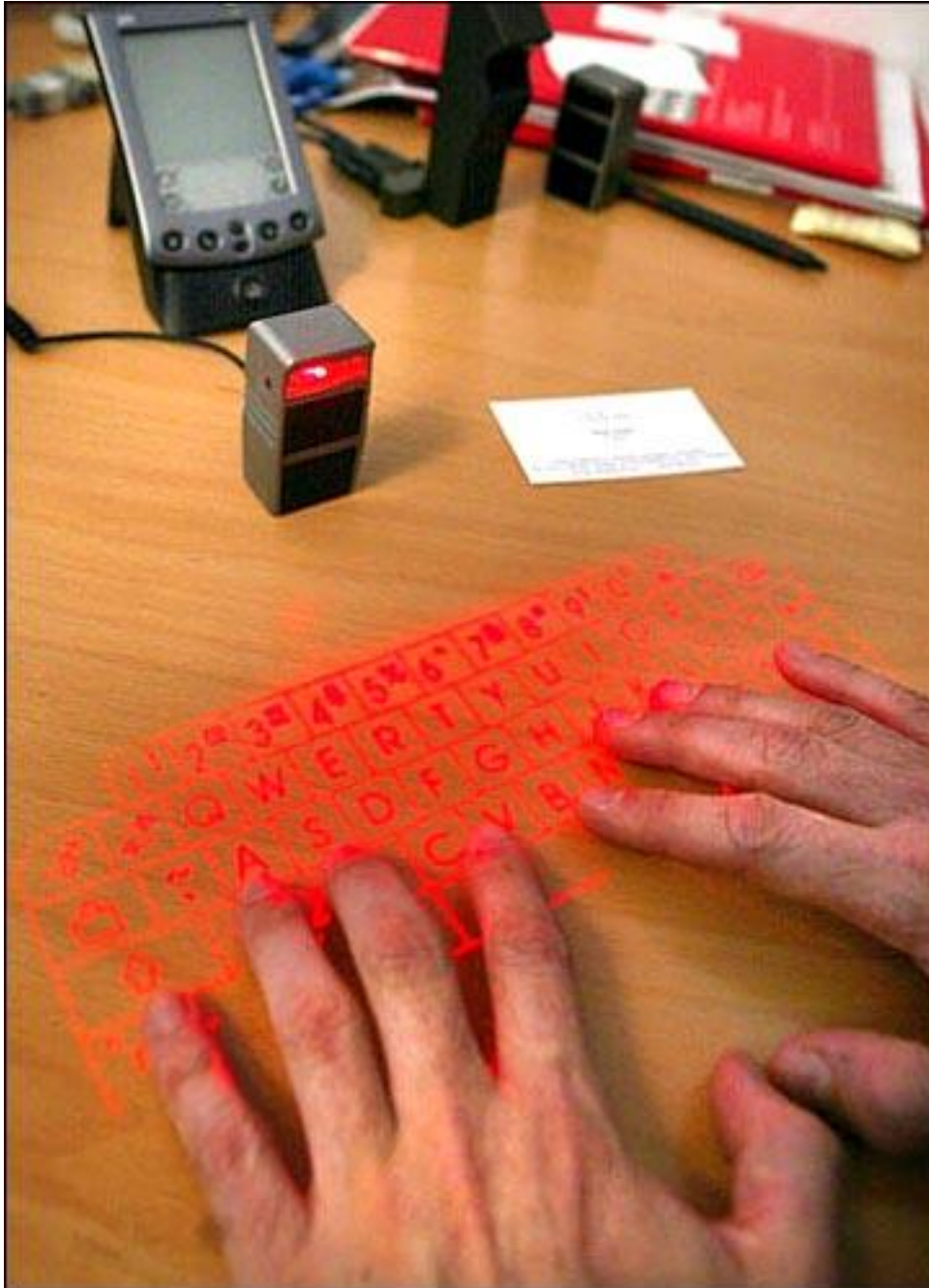
Figure 22: Another Virtual Keyboard: This unit was demonstrated by Siemens Procurement Logistics Services at CeBIT 2003 in Hanover, Germany. The technology was developed and manufactured by VKB Inc, in Israel. (Image: VKB, Inc.)
