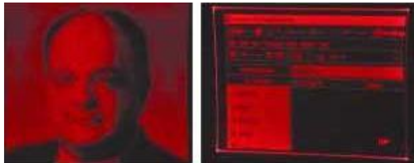
Figure 28: Example Output from Prototype Miniature Laser Projector. Monochrome images can be projected on arbitrary surfaces. Because the projector uses a laser, the images will always be in focus.
