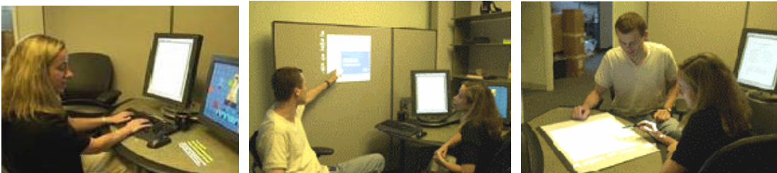
Figure 25: Bluespace: Reconfiguring Display Surface in Office Context. The same steerable projector-camera pair can direct the output display onto any number of different surfaces, including the desk, wall, and meeting table (as well as the floor, etc.). The user(s) can interact with the data displayed in any of the locations, by means of the camera. (Images: IBM)
