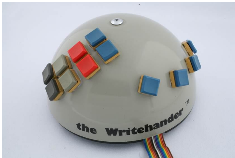
Figure 2: The Writehander (NewO Co.): a chording keyboard for one-handed text entry.
