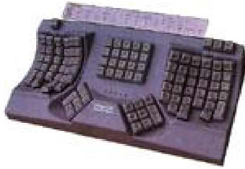
Figure 1: The Maltron keyboard: radical design sculpted to fit shape of hand and fingers.
