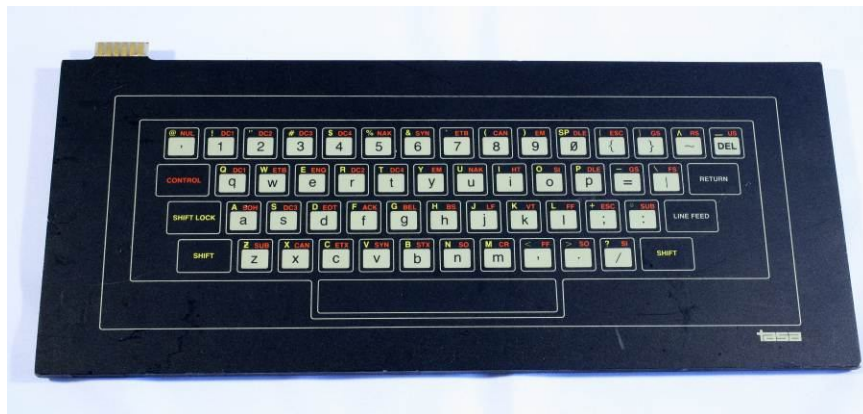
Figure 3: The TASA Keyboard: a touch-sensitive keyboard with no moving parts. Useful In environments which must be quiet (such as a recording studio), those which are very dirty (such as factories), or those which are very clean (such as hospitals).
