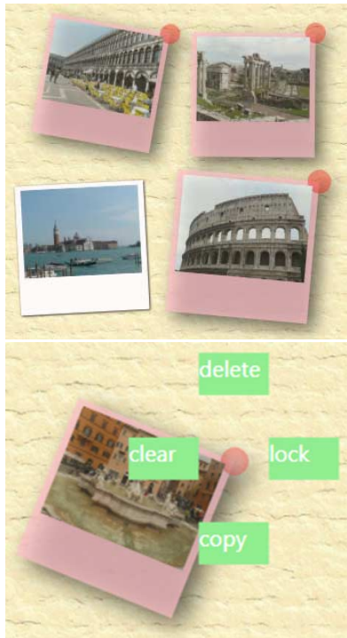
figure 4. Selection and Context Menu. (Top) Selection feedback consists of a pink highlight and a large drop shadow to visually “float” the object. Deselected objects have only a thin drop-shadow. (Bottom) Context menus use a radial (marking) menu. The user touches pen or finger to the red dot and strokes towards the desired command. This represents one situation where it is necessary to support both pen and touch interchangeably to match user expectations, even though elsewhere the system sticks to a differentiation of roles between pen and touch.
